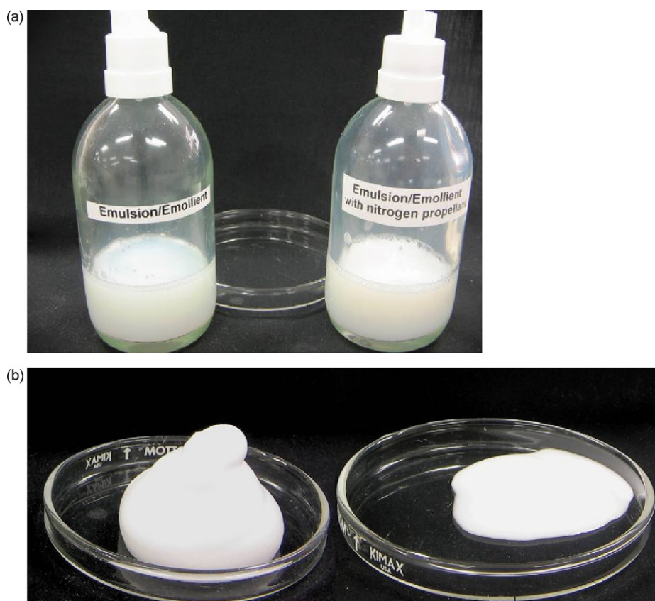
Fig. 6. (a) Emulsion aerosol base with hydrocarbon AP70 (left) or nitrogen (right). (b) Foams produced using hydrocarbon AP70 (left) or nitrogen (right).
