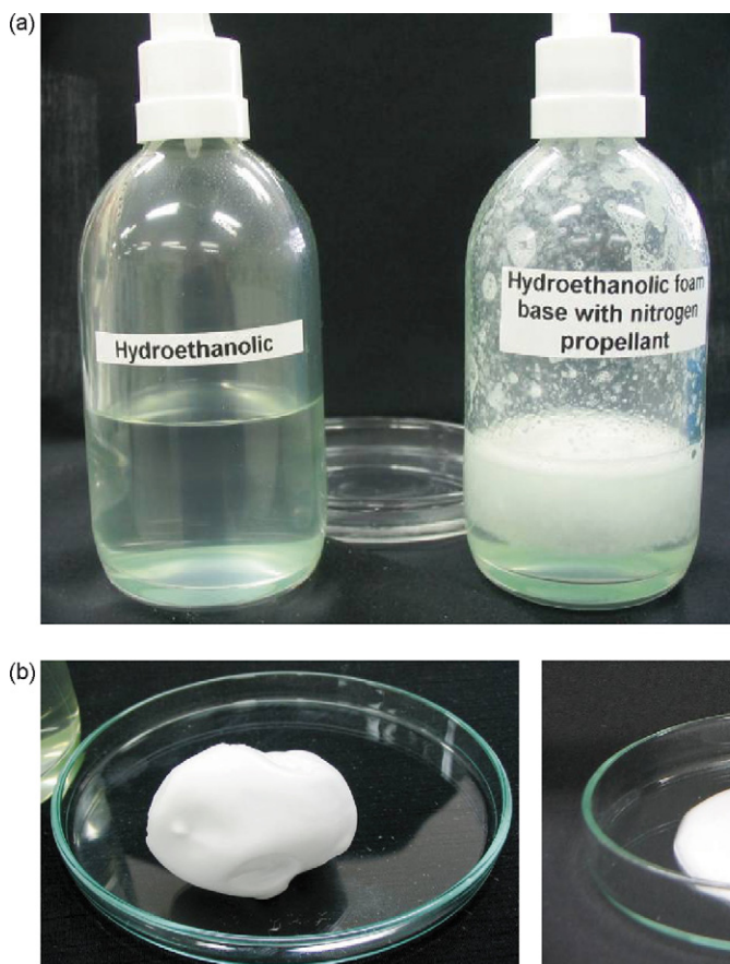
Fig. 5. (a) Hydroethanolic aerosol base with hydrocarbon propellant (left) and nitrogen (right). (b) Foam produced from hydroethanolic aerosol base with hydrocarbon propellant (left) and nitrogen (right).
